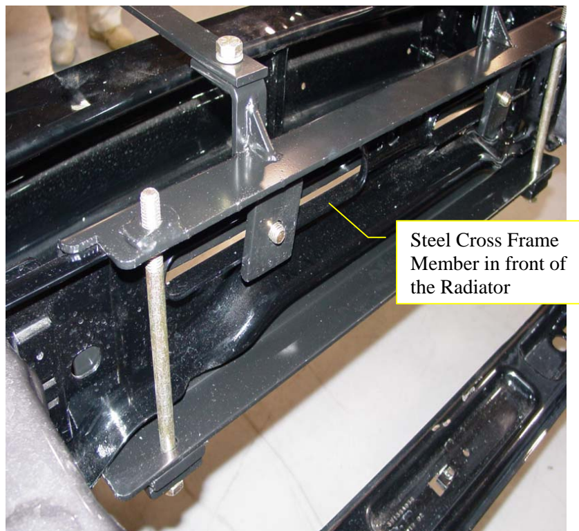
Photo 4 (Please note that photo 4 is taken of push bumper fully assembled to a chassis only.)
